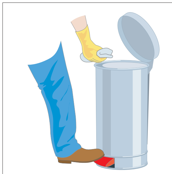
Figure 15: A fire-resisting pedal bin for rags
